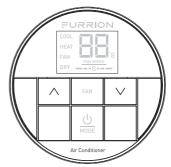
Simultaneously press both  $\land$  and  $\lor$  buttons for 3 seconds to toggle the temperature format between Centigrade and Fahrenheit.
