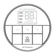
After the thermostat is turned on, press button repeatedly to toggle through the available modes. The activated mode icon and temperature set-point will be displayed on the LCD. The thermostat will transmit the last selected operation mode command to the control box after 2 seconds without any operation.
