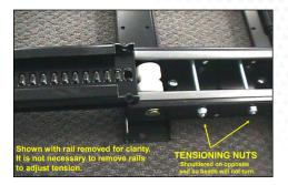
To minimize slider "creep". These tensioning nuts can be tightened. Tighten these nuts in small increments until you just begin to hear a change in the motor pitch, indicating that the moving tension of the rails has been slightly increased.
