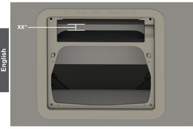
**4.** Cut and remove an amount of the top insulation foam divider equal to the recorded measurement height.
