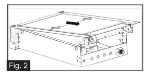
3. Slide the hob into the cabinet opening. Verify the hob is level from side to side and front to rear. (Fig. 3)
