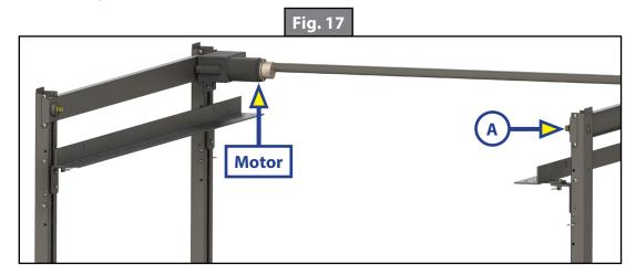
**E.** Using a socket wrench, move the non-motor side to the desired height (1/4" to 1/2" higher than the motor side) and hold at that position while the cross-connecting shaft is reinstalled.
