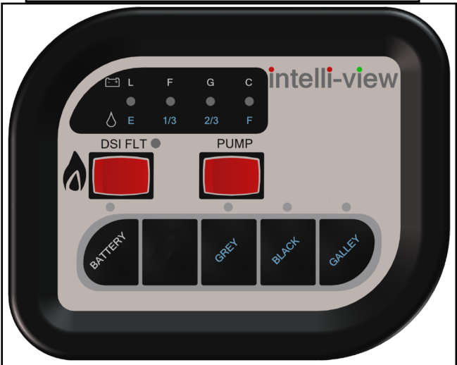
Fig. 4 - Three Tank With Two Switches
