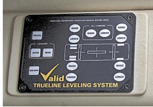
Mounted control panel
