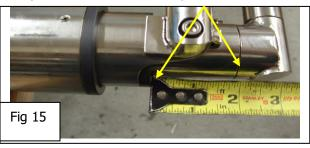
With the crossbars disconnected, adjust the tubes by turning off the power to the unit and rotate the tubes to match each other in extension. Rotating the tubes clockwise will screw the tube into the stationary tube (reducing the length) and counterclockwise rotation will screw the tube out of the stationary tube (increasing the length). Once both actuators are at the same length, reassemble the crossbars and power.
