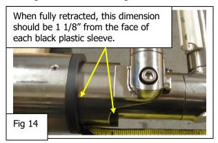
When fully retracted, this dimension should be 1 7/8" from the end of the tube (not including the crossbar insert) to the face of the black plastic sleeve.
