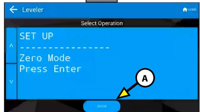
5. The touch panel will present options for further leveling of the trailer if needed. The screen will also state "ZERO POINT CALIBRATION - Press Enter to set" (Fig. 9).
