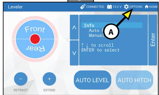
4. The touch panel will present options for further leveling of the trailer if needed. The screen will also state "ZERO POINT CALIBRATION - Press Enter to set" (Fig. 4).
