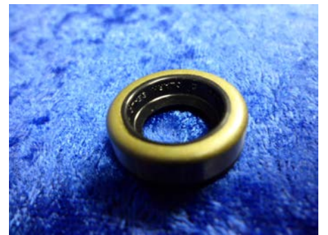
Figure 9 Close-up of the shaft seal (030-1071). Metal side goes in against the port plate.
