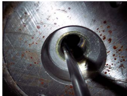
Figure 8 Punch out seal from motor side of the port plate
