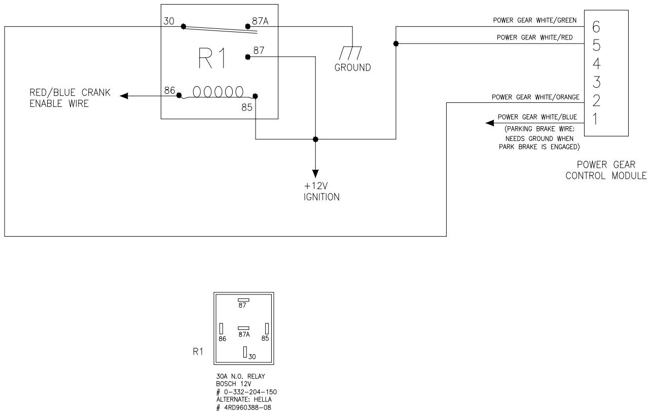
Wire up the Power Gear control as shown in the schematic above. Test the control by extending the jacks and releasing the park brake. Also extend the jacks and put the coach into gear. The alarm should sound and the jacks should automatically retract in each case.
